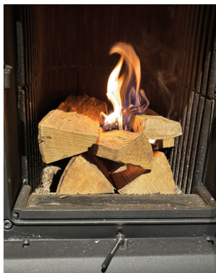
Arrangement of lighters, kindling sticks and logs for heating from above
